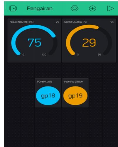
Gambar 18. Media *Interface Blynk* Sistem Pengairan
