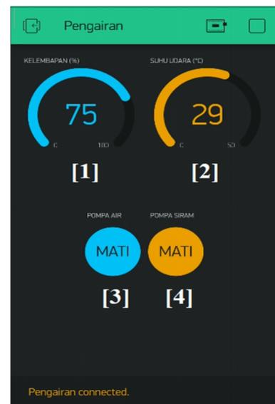
Gambar 19. Media *Interface Blynk* Sistem Pengairan
