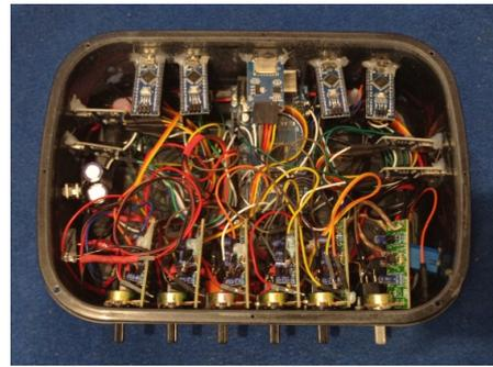
**Gambar 6:** Module Pad Trigger Rebana Tampak Atas
