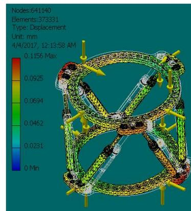
**Figure 14.** Displacement is on the external frame fixation with standard components.
