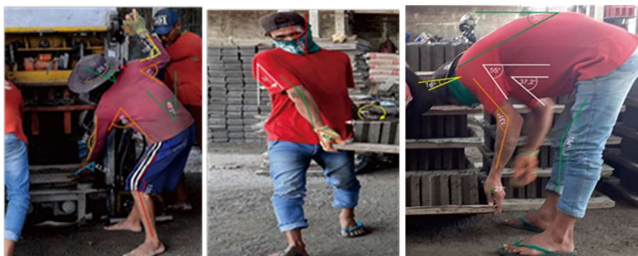
Figure 2. The activity of Lifting, Transporting and Laying of Molding Results.
