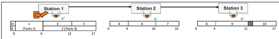
Figure 5. Scenario 2a: Setup time = 1.
