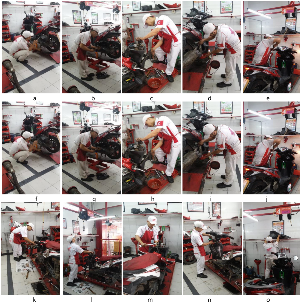
(a) open the back machine, (b) open the back machine on the pit, (c) assemble the motorcycle's handle using hammer, (d) change the oil, (e) inject the fuel, (f) check the chassis, (g) check the fuel injection, (h) fix the chassis, (i) fill in the water coolant, (j) open the underparts of the machine, (k) fix the chassis, (l) gain the hanging tool, (m) assemble the chassis, (n) assemble the handle of the motorcycle, (o) take off the seat
