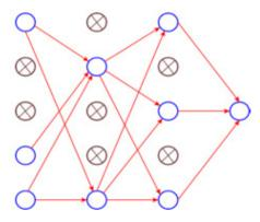
Figure 8. After Applying Dropout
