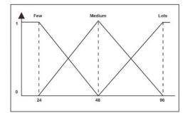
Figure 6. Graph of Membership Functions variable number of error points at medium level
