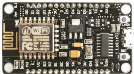
Figure 7. Composition of pins on NodeMCU + ESP8266 [20]
