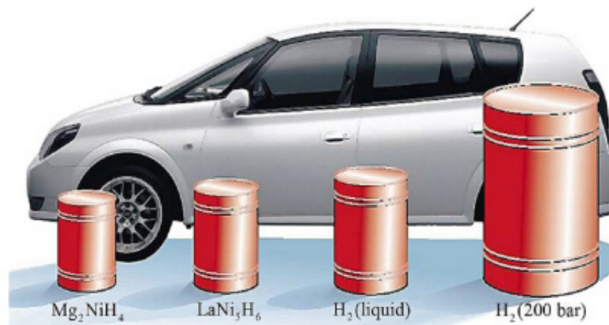
Figure 1.1 Volume of 4 kg of hydrogen compacted in different ways, with size relative to size of a car (Image of car of Toyota press information, 33rd Tokyo Motor Show, 1999 [5]).
