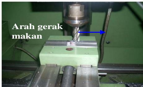
Gambar 5. Proses down Milling
