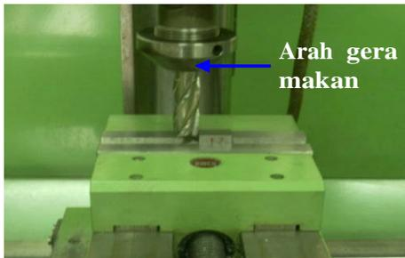
Gambar 4. Proses up milling
