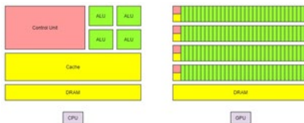
Figure 1. CPU and GPU architecture design illustration
