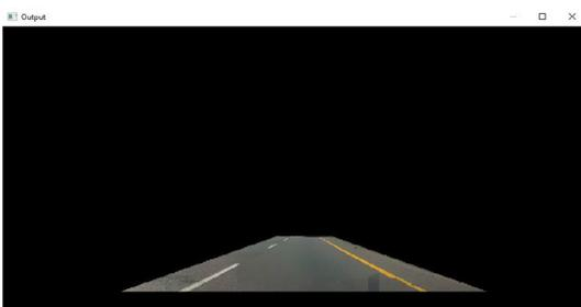
Figure 4. Display a frame with ROI and mask
