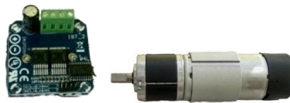
Figure 9. Driver Motor 43A BTS7960 IBT2 and Motor DC PG 28 + Encoder 7ppr
