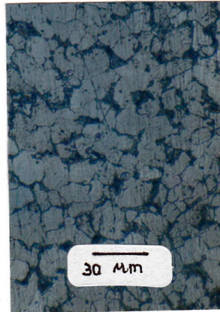
Figure 1. Microstructure of the raw material
