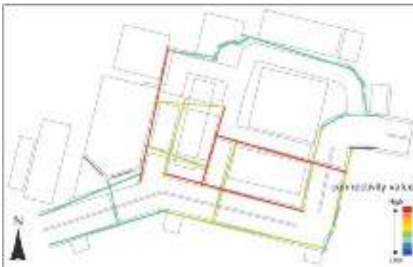
Figure 14. The axial line for the connectivity value of the pedestrian segment around the Planetarium building (Source: Author Analysis, 2022)
