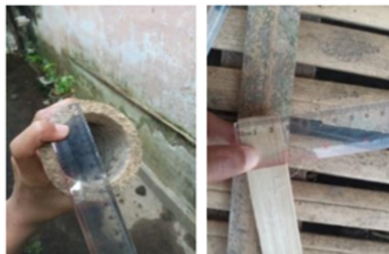
Figure 2. (a) Measurement of the Diameter of Bamboo to be Used as Puppet Material; (b) Measurement of the Width of Bamboo Splits After Splitting One Bamboo Lodge into 8-10 Parts (Researcher Documentation)
