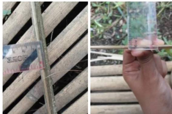
Figure 3. Measurement of Bamboo Split Thickness (a) Before Drying and (b) After Drying (Researcher Documentation)
