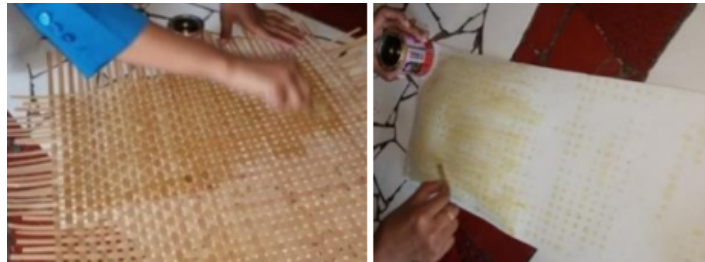
Figure 6. Process of Applying Glue to Strengthen Woven Bamboo and Sponge (Researcher Documentation)
